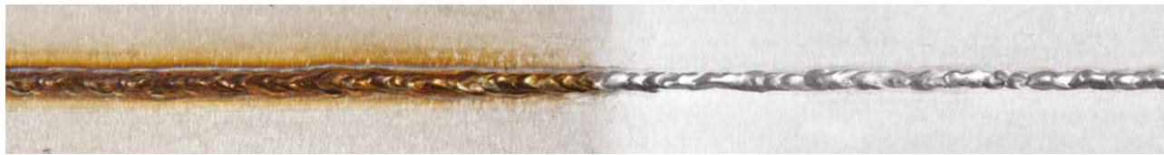
TIG welding in two steps
